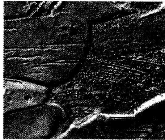
Figure 8. Deformation twins present on the cross section of the tantalum sample spalled at 17 GPa shock pressure.
